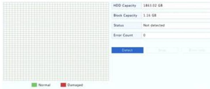
2. Select the desired disk and detection type, and then click **Detect** to start detection. Click **Stop** if you want to stop.
