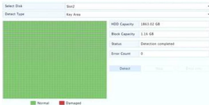
Note: The detection stops automatically when the error count reaches 100.
