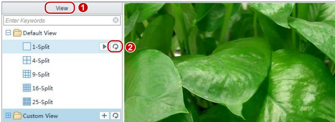
After sequence display is enabled for a default x-split view, the live videos of cameras in the camera list are played by turns in x windows.
